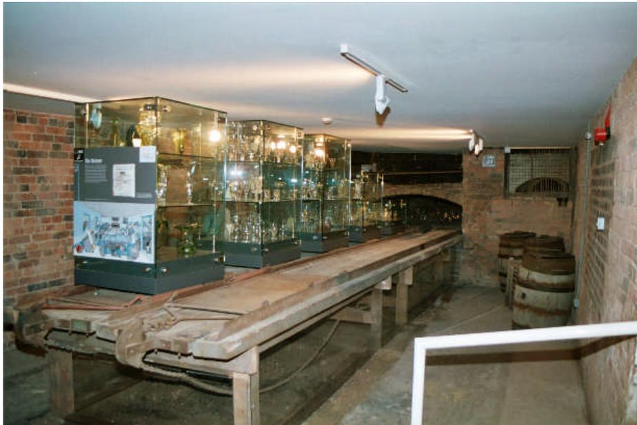
**Figure 3.13: 'Delivery' end of an annealing lehr (Red House Cone)**
