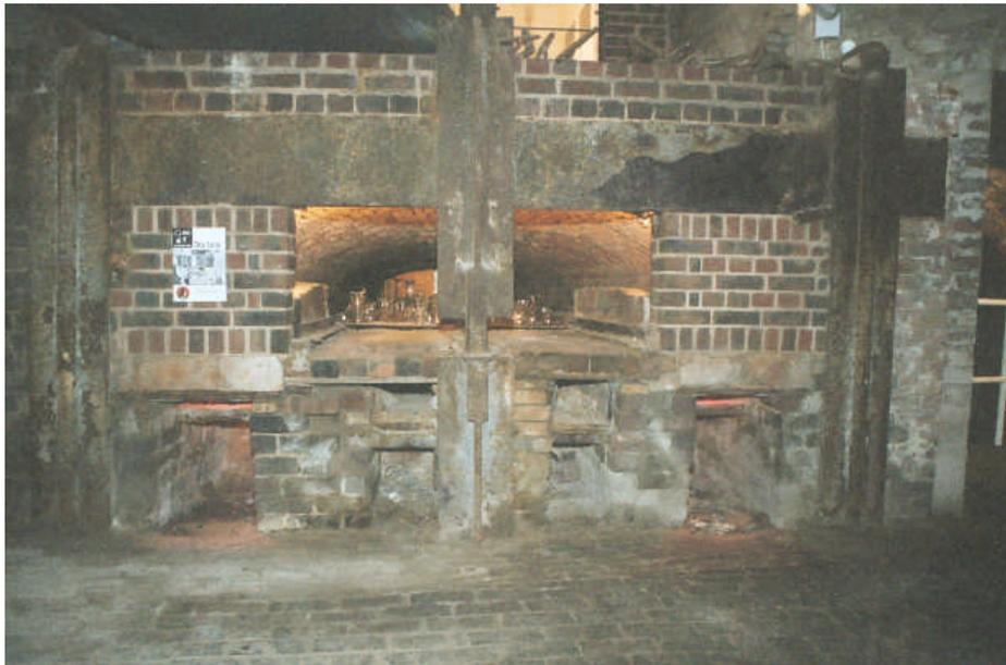
**Figure 3.12: 'Input' end of an annealing lehr (Red House Cone)**
