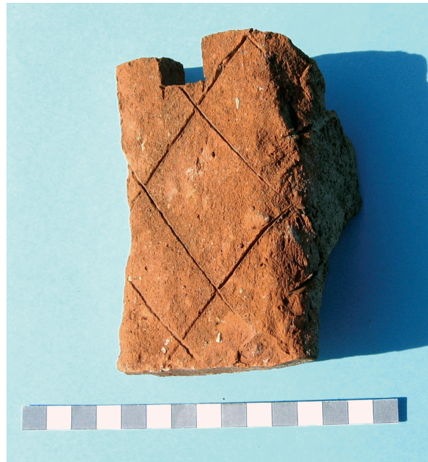
Fig. 1: tile type 1, showing lattice-scored narrow face with vent (WP83 [1613]).
