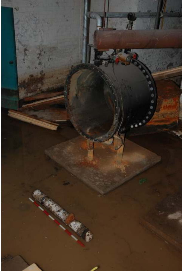
Fig 15 The location of the drilled core through the concrete slabs in the area of Trench B. The borehole can be seen to the left of the 1m scale. The core of concrete measured 1m and beneath this was a further c 250mm of loose concrete. Therefore the total depth of the concrete slabs in the location of Trench B is 1.25m and assuming the top of the basement floor to be at c +0.582m this gives a reduced level for the base of the concrete in Trench B to be at -0.668m OD.
