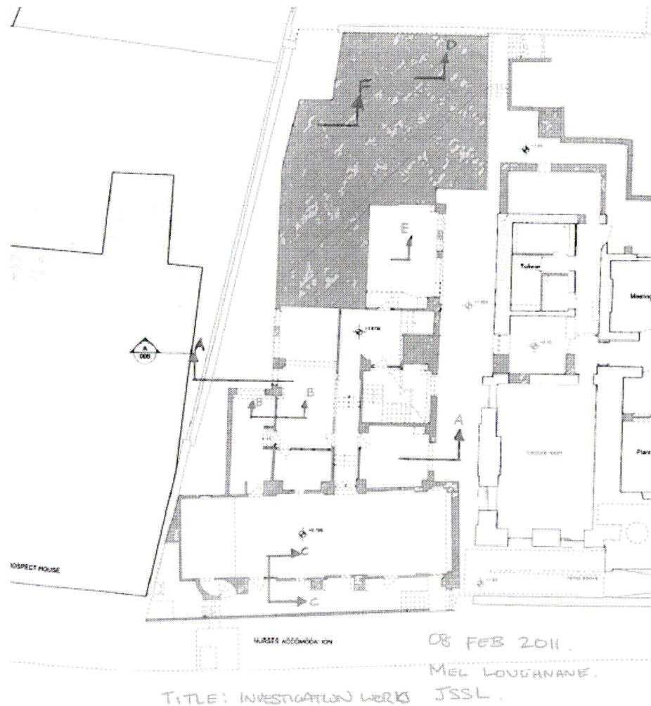
Fig 5: Plan of the site showing location of slab thickness profiles, see Figs 6 to 8 for sections. © John Sisk & Son Ltd. 2011.
