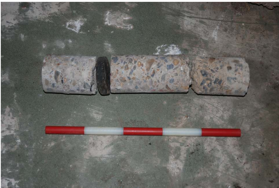
Fig 21 The core from the lower slab in Trench C, part of this core could not be retrieved and the actual core was 700mm in depth, with 250mm of loose concrete below (Scale:500mm).
