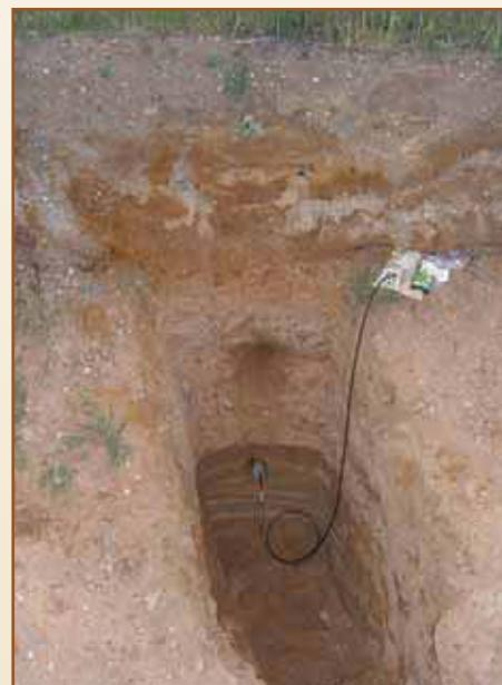
*OSL field technique: a gamma spectrometer measuring the natural radiation present in a Quaternary sediment*
