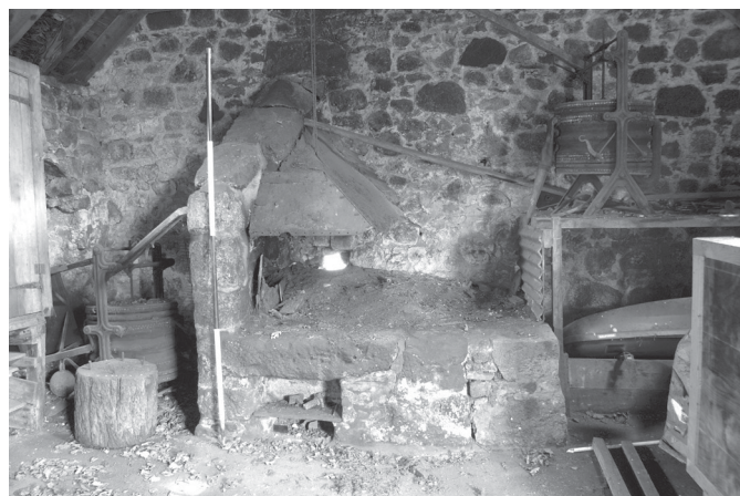
Glen Dye Steading: the forge with original bellows
