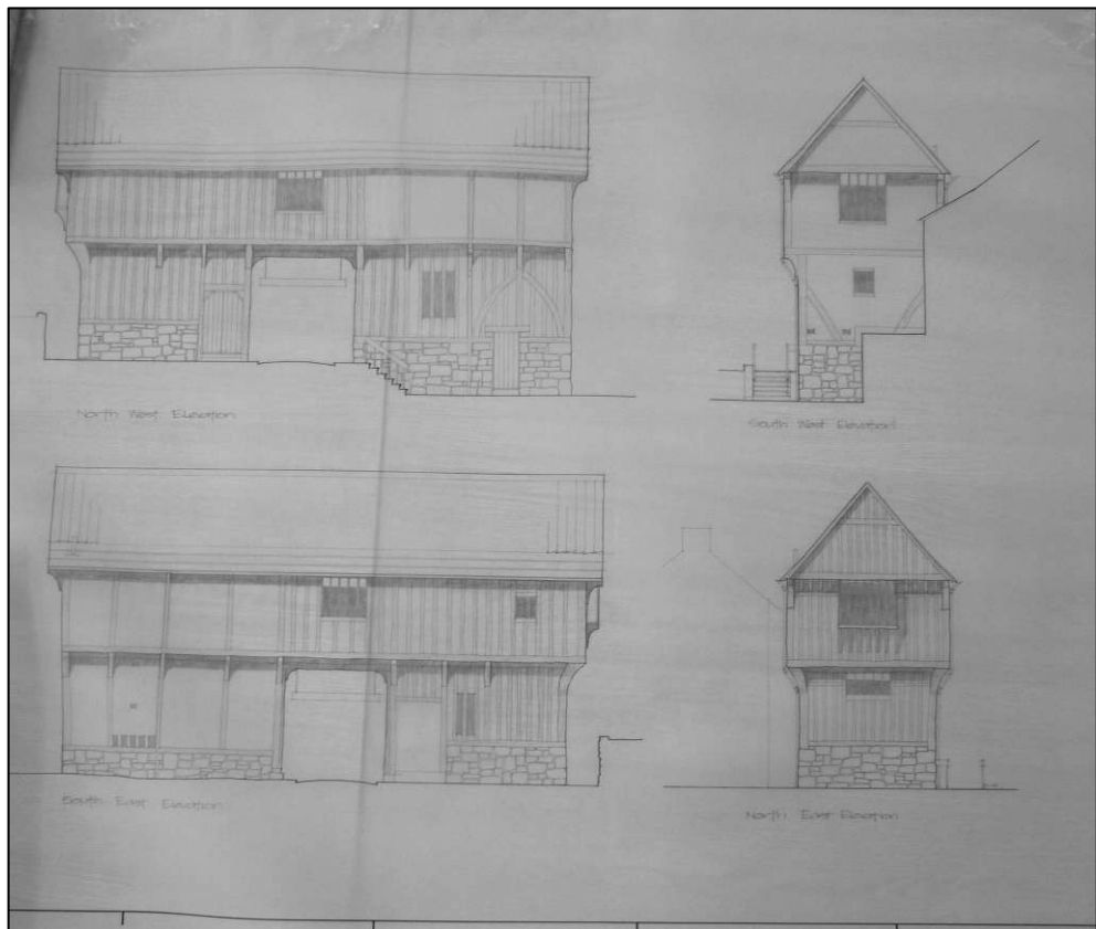
Plate 4: Brierley, Leckenby, Keighley & Groom's sketch design for the complete restoration of the gatehouse, November 1979 (York City Archives B46/1 shelf O4F).
