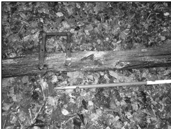
Photo 2/468: Timber 2 - detail of wrought-iron brackets.
