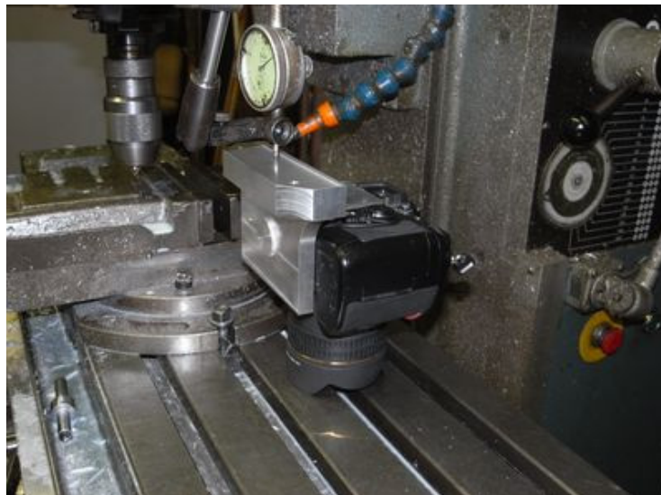
Figure 51. Manufacturing of Camera support for the Housing
