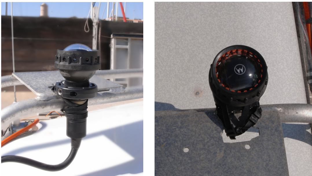
Figure 14. SOSI Series GPSR-X015G Satellite Differential GPS Receiver mounted on the Remora 2000.
