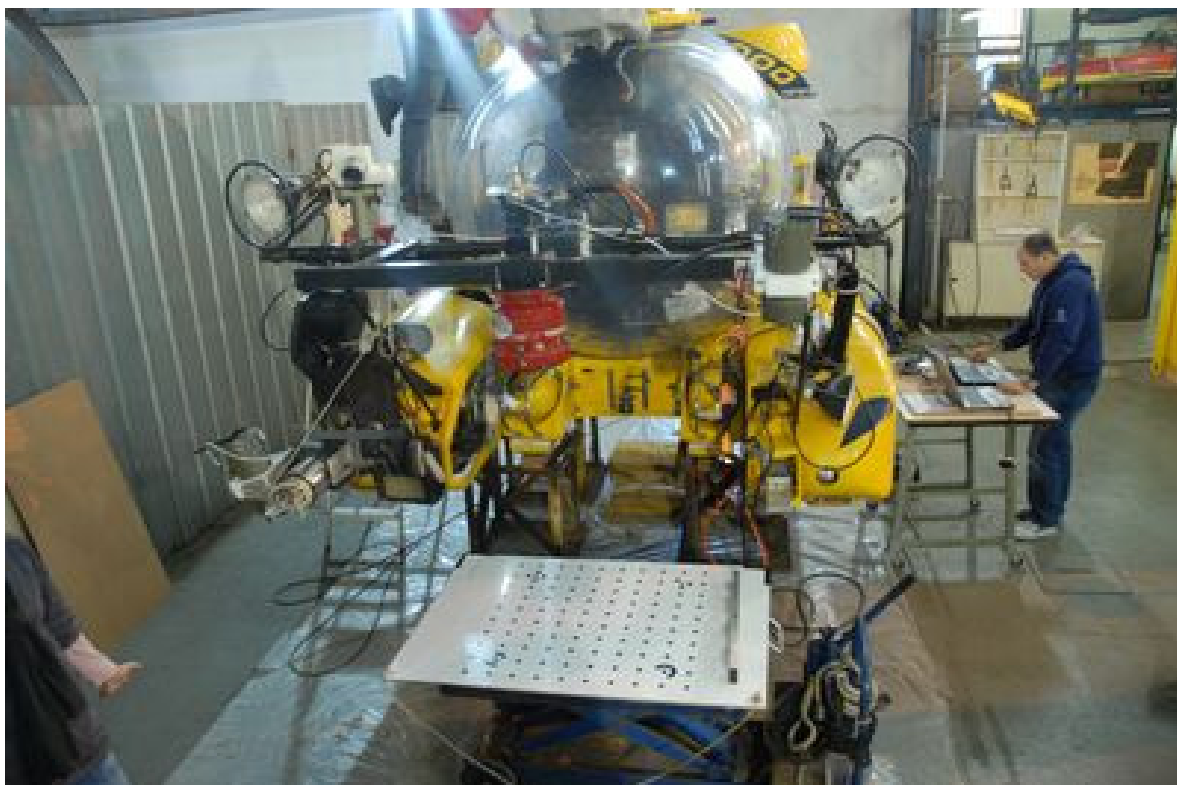
Figure 53. Calibration grid leveled under the Camera.
