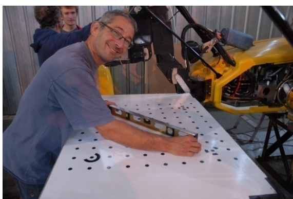
Figure 54. Setting the calibration grid horizontally. On the left: adding the PHINS sensor..
