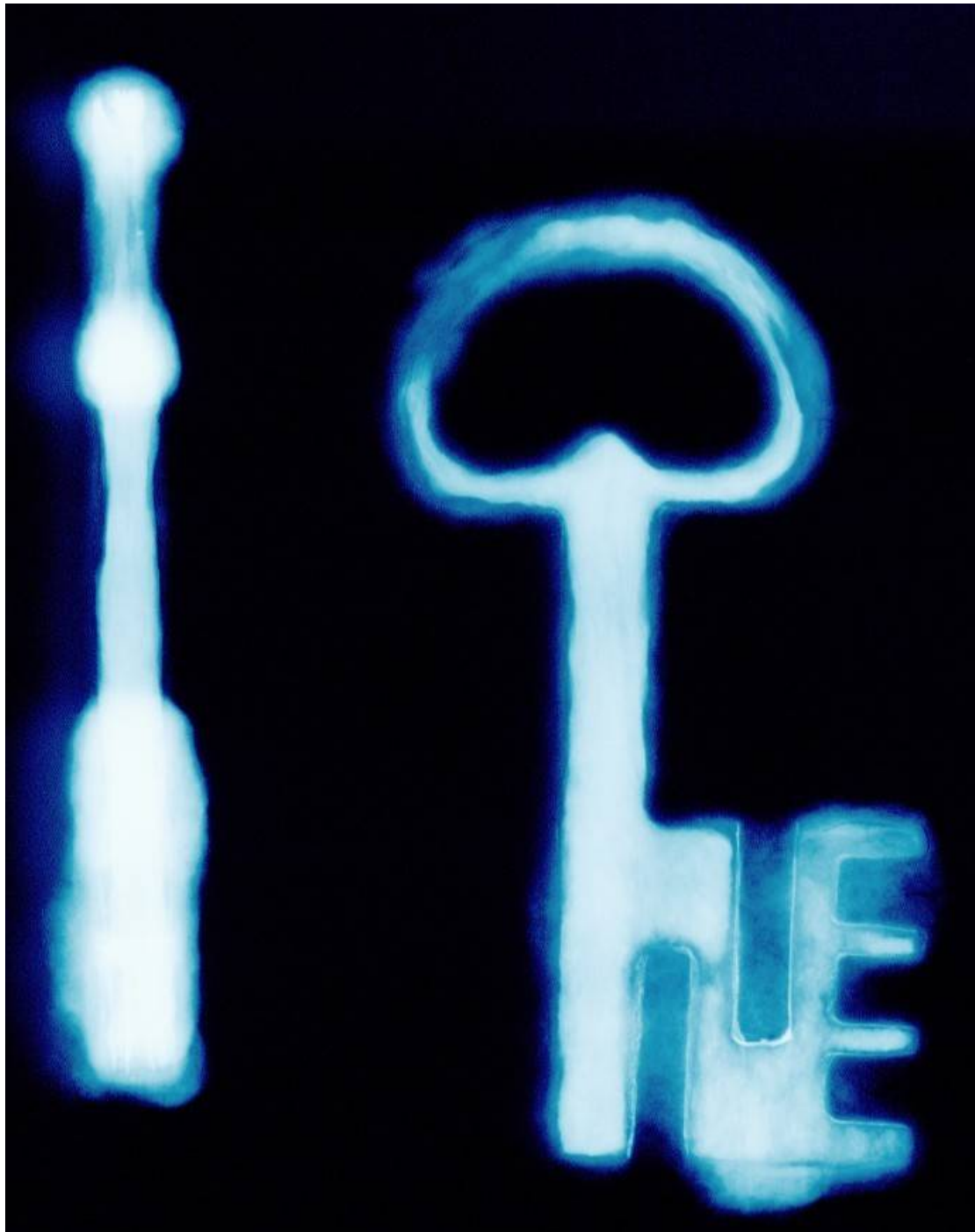
Figure 5 X-Radiograph of iron key, SF16
