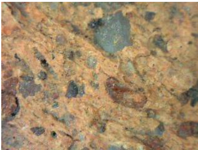
Figure 3 close-up of brick fabric showing coarse quartz, sandstone and ironstone sand
