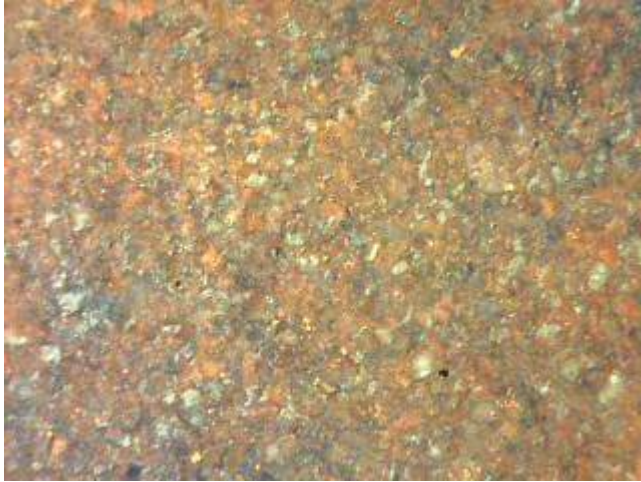
Figure 6 moulding sand on pantile
