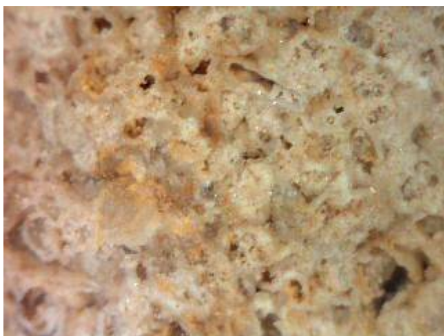
Figure 1 Close-up photograph of freshly broken edge of stone (width of field of view c.3.4mm)
