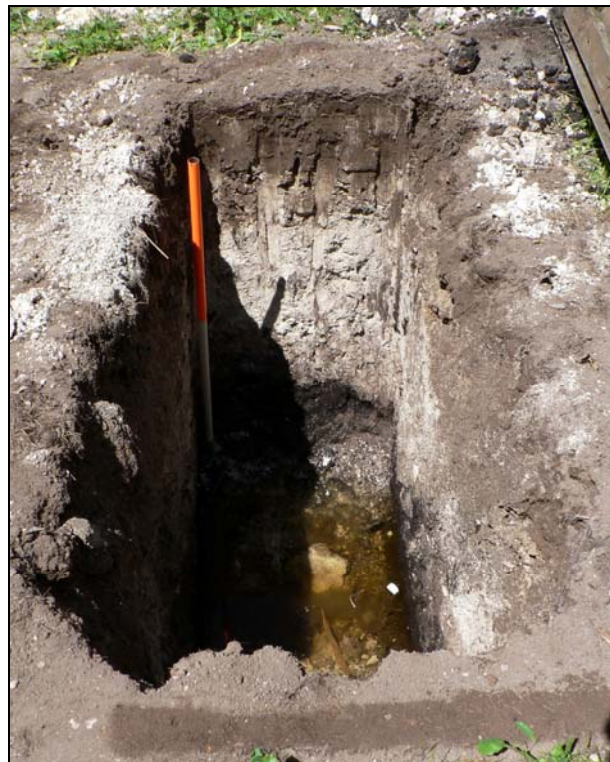
Test pit from east with chalk layer over peat
