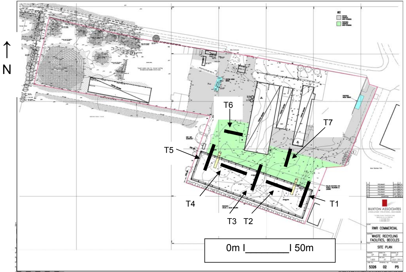
Proposed trenching plan (5 x 30m & 2 x 20m)
