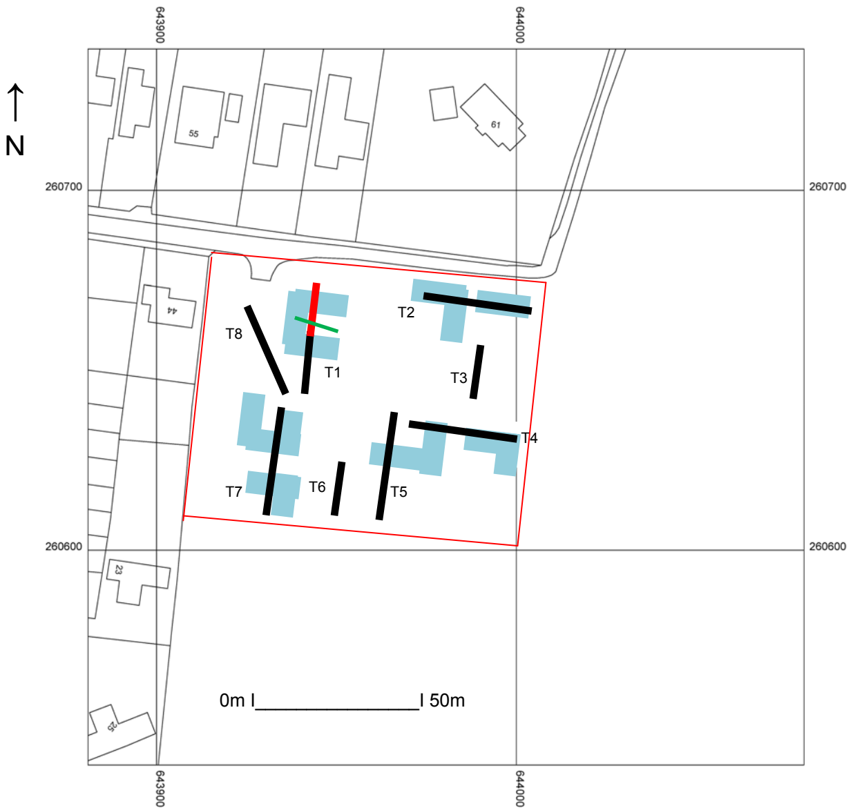
Fig. 2: Location of trenches (trenches 3, 6 & 8 in areas of access/parking) (Light blue- Planned house footprints, red- see Fig. 3, green- ditch 0004) (Ordnance Survey © Crown copyright 2015 All rights reserved Licence No 100049722)
