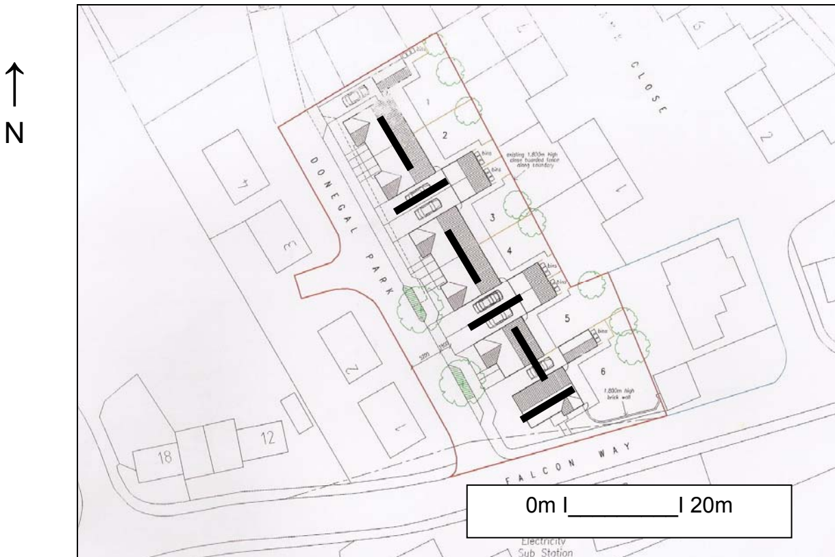
Proposed location of trial trenches (6 x 10m each)
