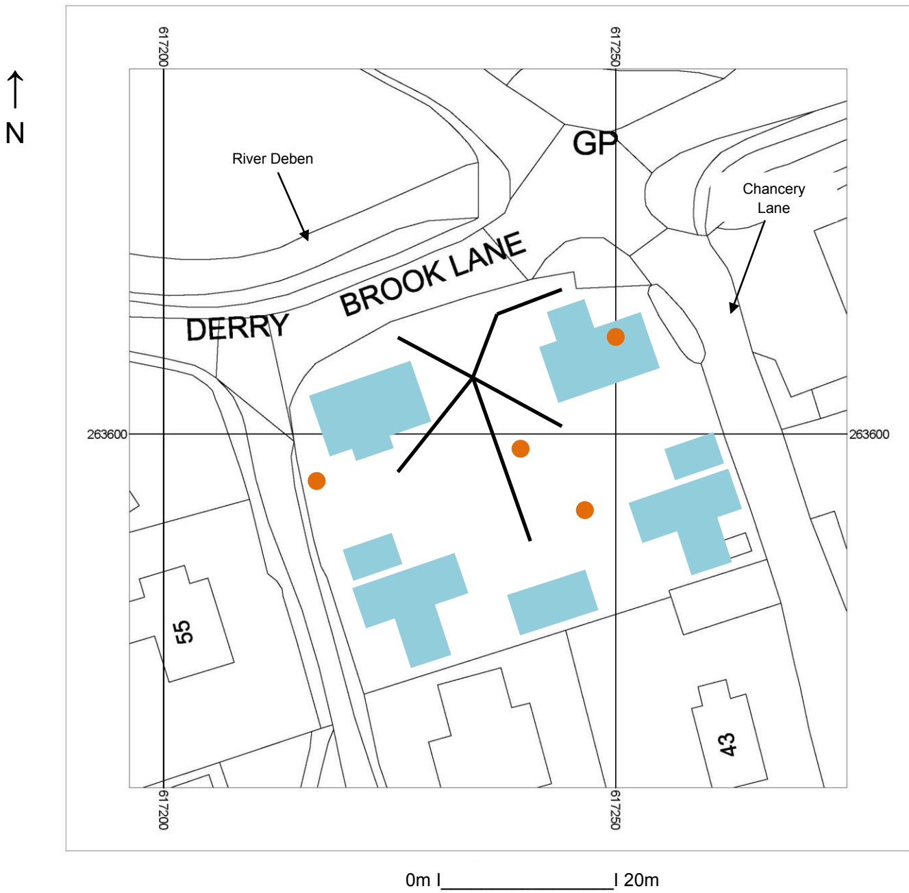
Fig. 2: Location of monitored areas (light blue- footprint areas with shallow soil strip, black lines- drainage trenches, brown- old fuel tanks)
