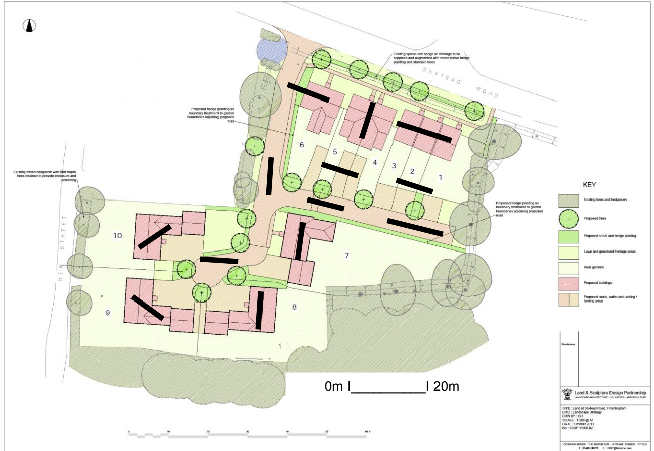
Proposed location of trial trenches (11 x 10m and 2 x 15m)
