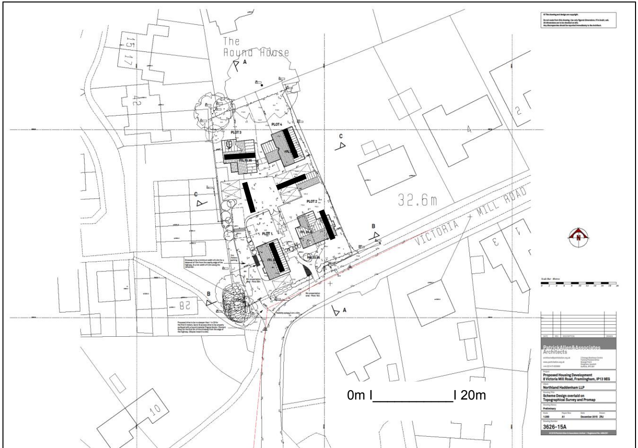
Proposed location of trial trenches (6 x 8.30m and 10m left as contingency)
