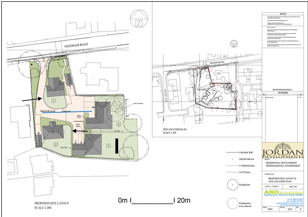
Proposed location of trial trench (1 x 10m) and foundation trenches to be monitored (arrowed) and gas pipe trench (blue)
