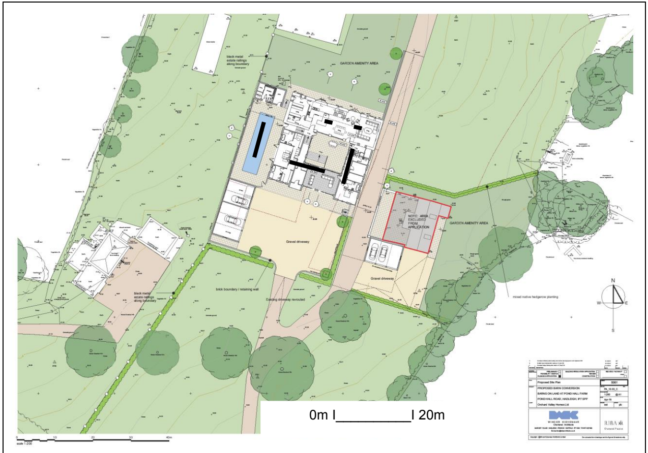
Location of trenches (3 x 8m) and approximate location of test pits
