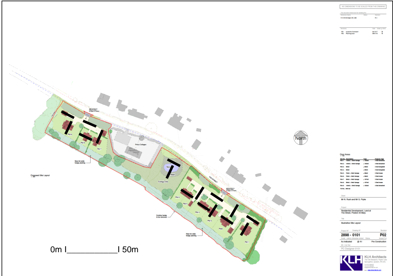
Proposed location of trial trenches (16 x 15m plus 10m contingency)
