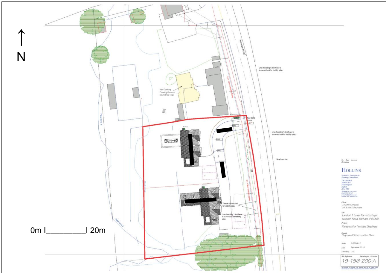
Proposed location of trial trenches (2x 10m & 2 x 20m plus 20m contingency)
