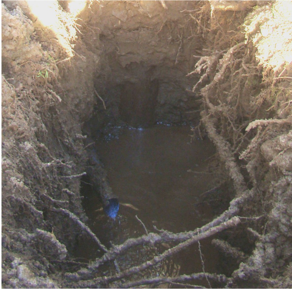
Figure 5a – Pit (2) showing groundwater level (from SW)
