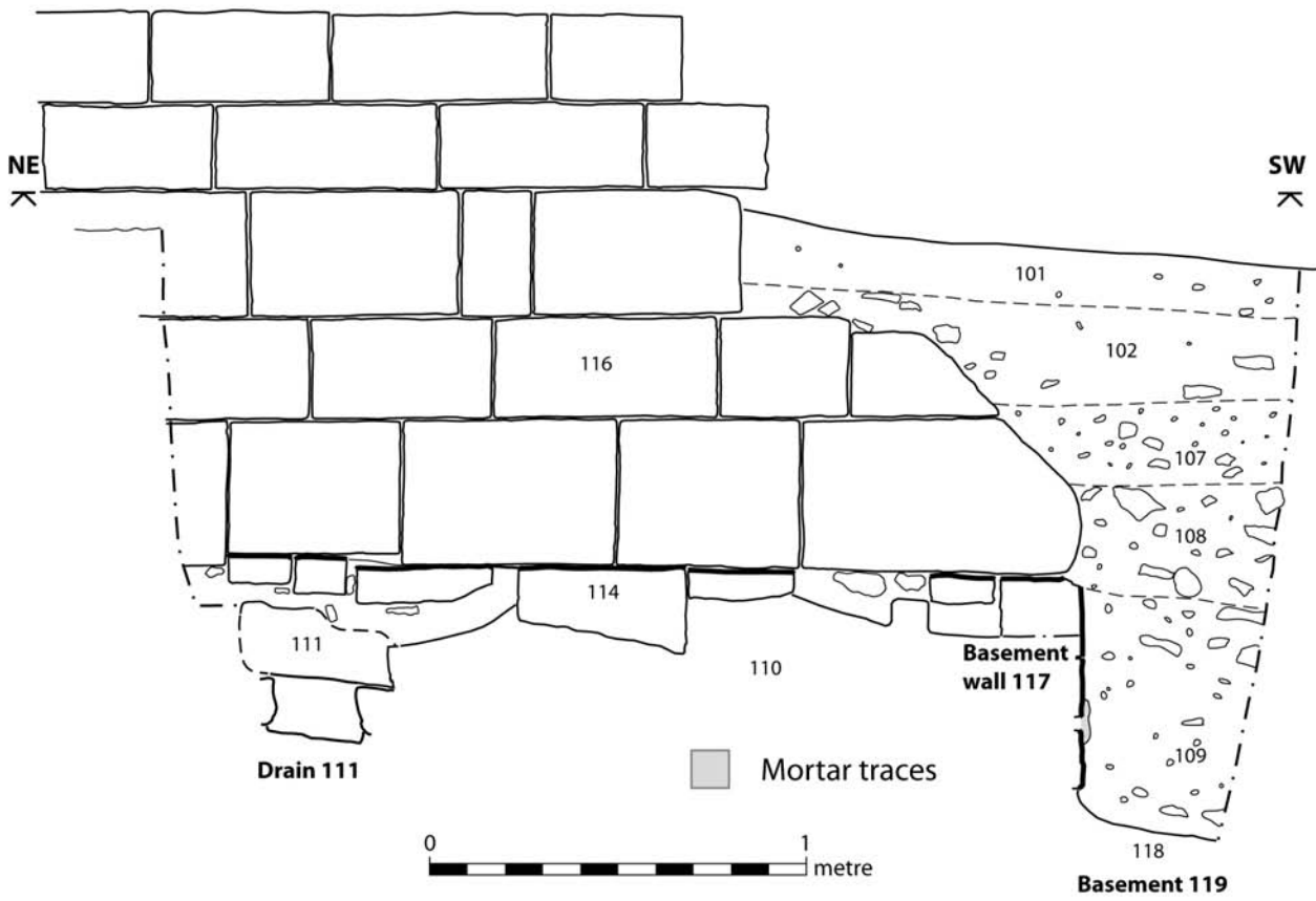
Figure 8: Elevation of southeast side of passageway.
