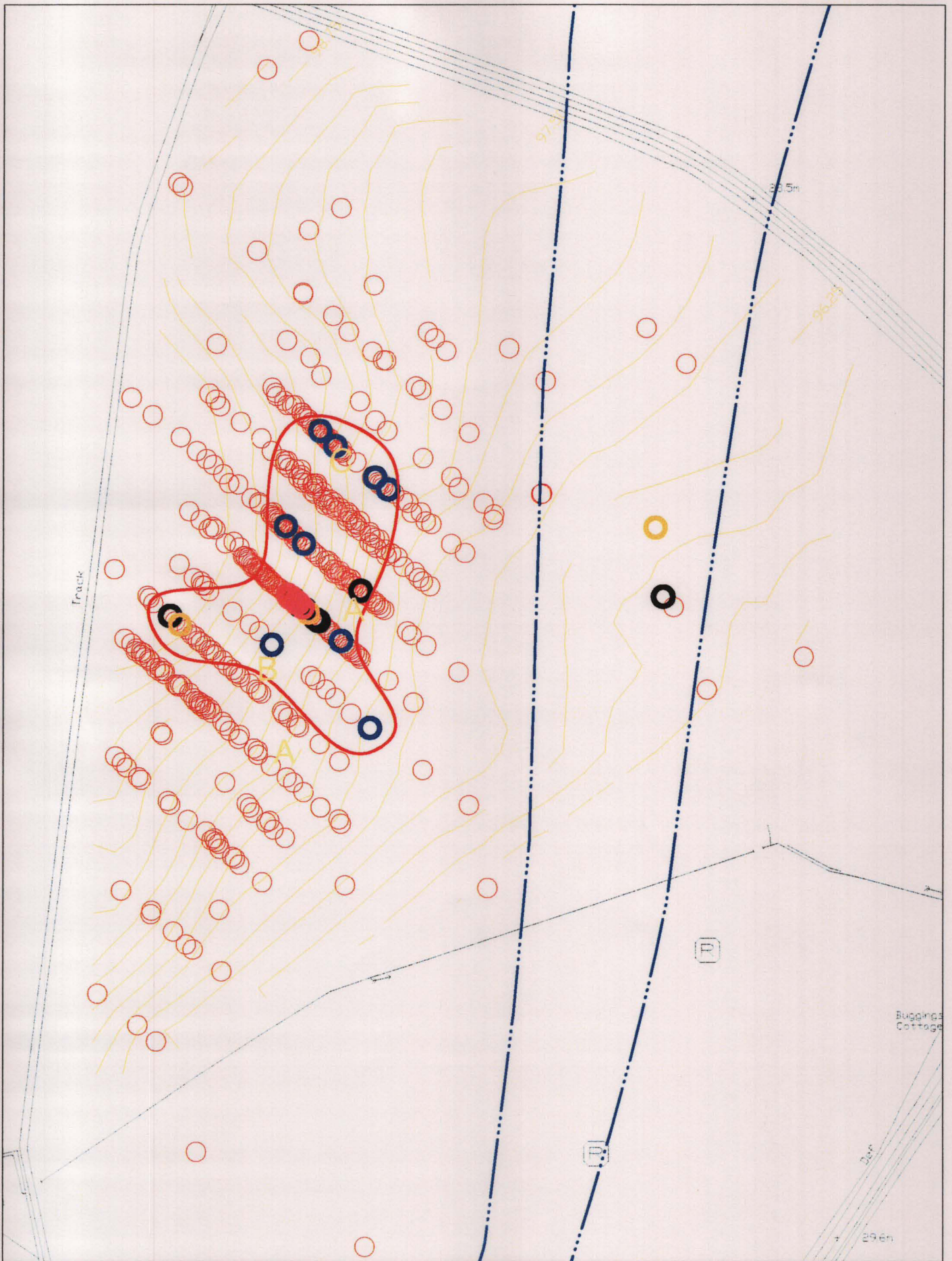
Fig. 10: Details of field 4437b showing off-line route (blue) in relation to distribution of Romano-British brick/tile (brown), concrete (yellow) opus signinum (pink) plaster (black) and slate (blue) scale 1:2,000
