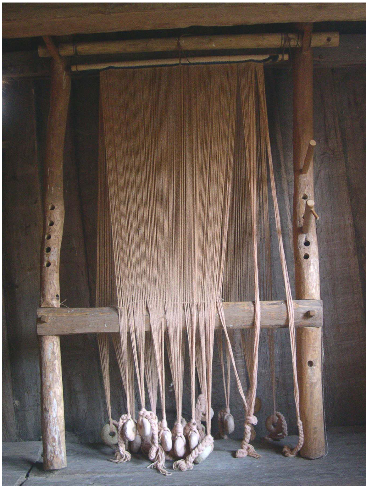
Reconstruction of warp weighted loom. Note the doughnut shaped loom weights keeping the warp taut
