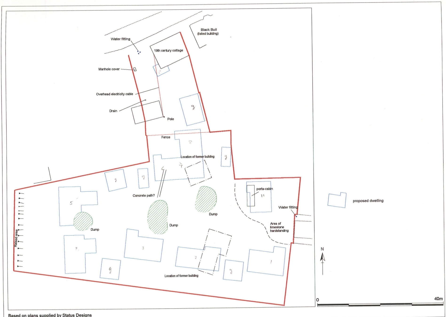
Figure 11 - Plan of the proposed development area, showing constraints and results of the walk-over survey
