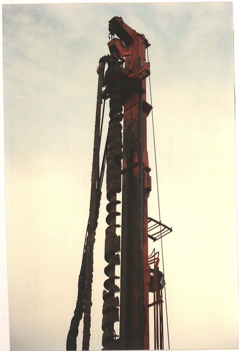
Pl. 13 Auger arm of Soilmec drilling rig showing concrete feed hose attachment at top centre of auger
