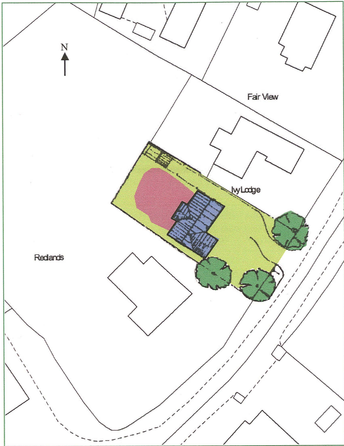
Fig. 2: Location plan of development plot, showing property boundary and house footprint. The area of the depression at the back of the property is shown in purple. Scale 1:500
