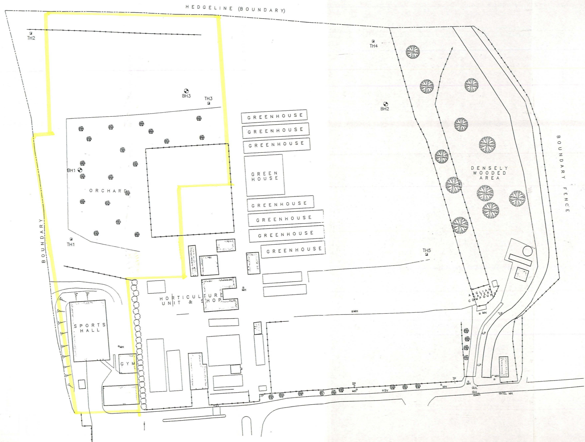
Fig. 2 The Application Site, showing existing structures and the position of recent trial pits and boreholes (reproduced from Alan Wood and Partners dwg. no. 21622/08A).
