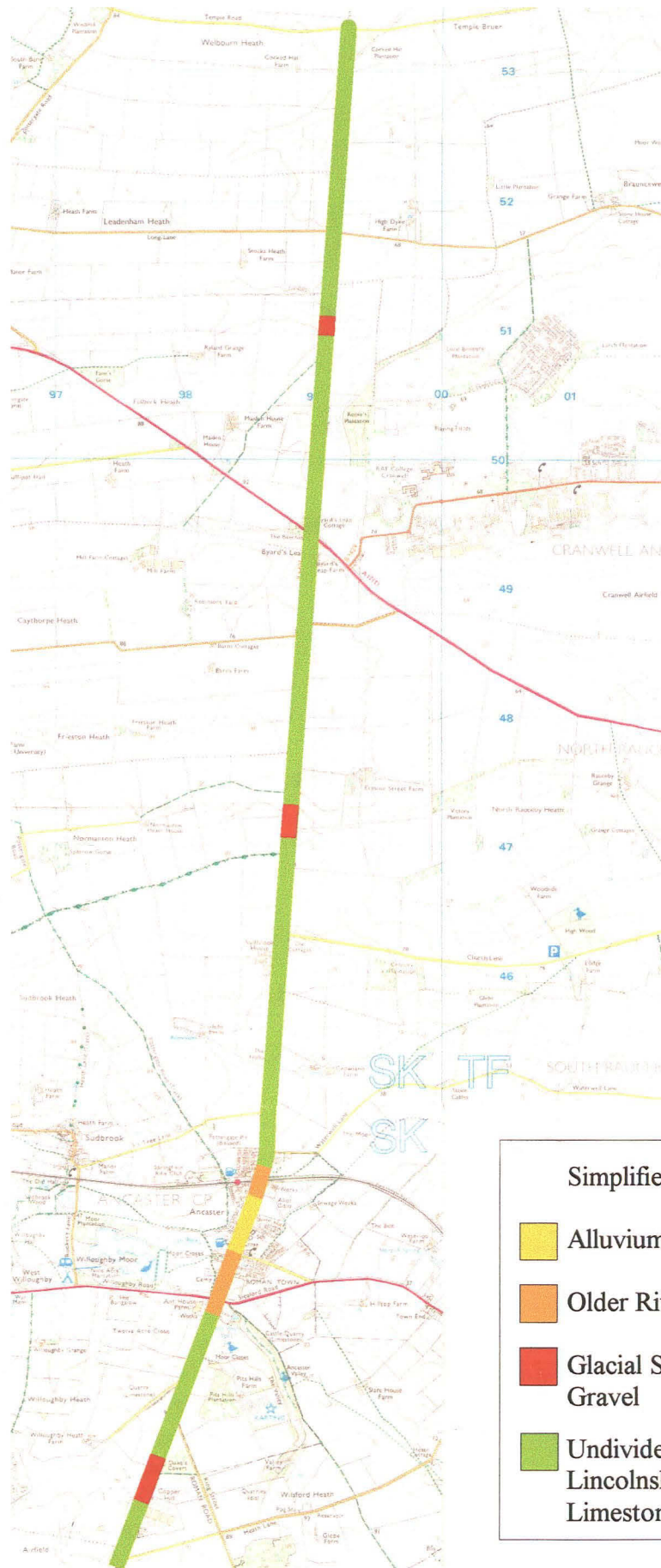
Figure 2: Simplified drift and solid geology of the pipeline route at scale 1:50,000. Note Lincolnshire Limestone is the overall solid geology. (OS Copyright Licence No: AL 515 21 A0001)
