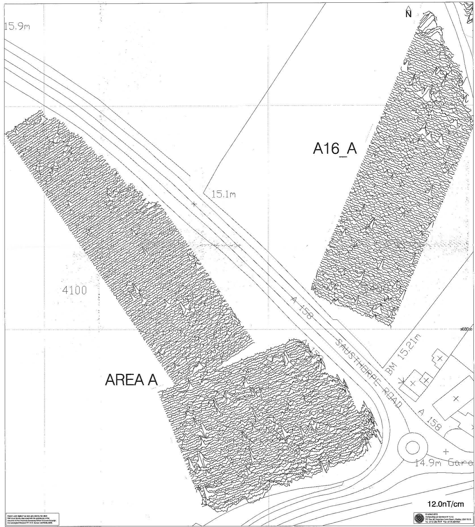
A16 - A158 Partney Bypass, Lincolnshire X-Y trace plot of the unprocessed gradiometer data; Area A and Block A16_A (1:500)
