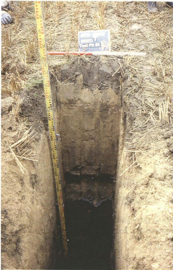
Plate 1: Section of Test Pit 60 within 'high silt' zone showing sticky blue clay overlain by silts.
