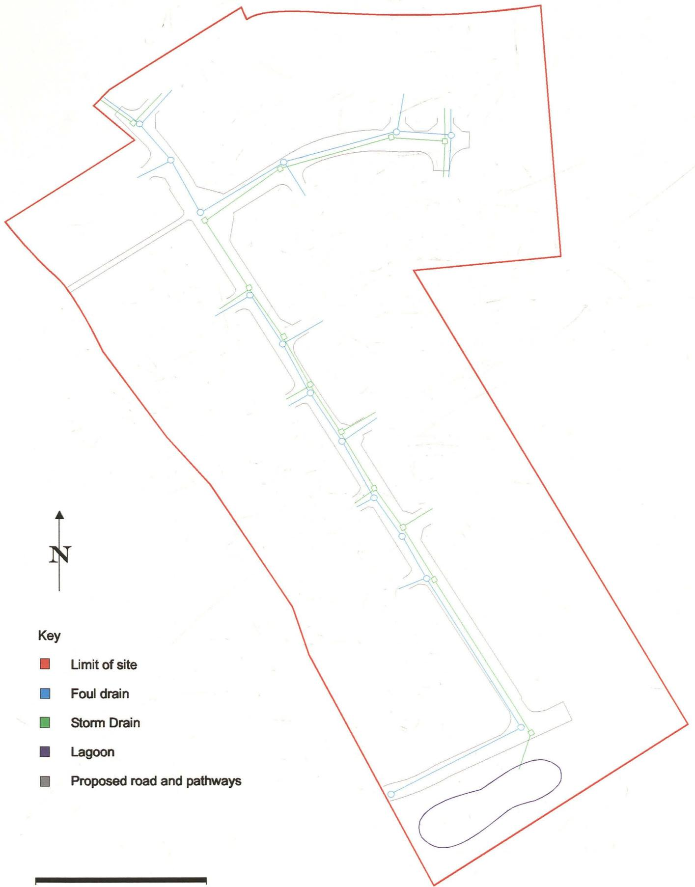
Fig. 2 Map of groundworks (after plan supplied by client)
