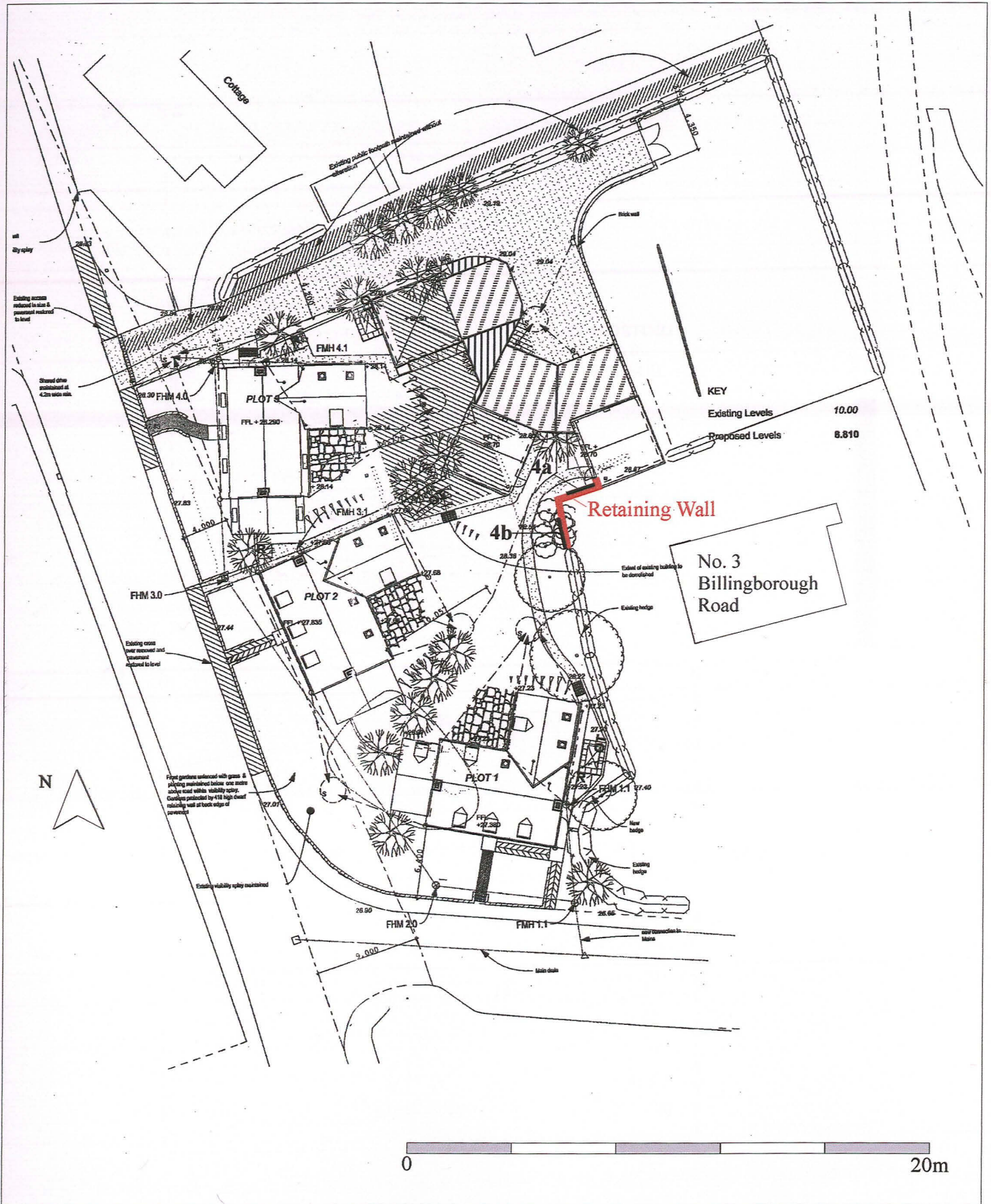
Fig. 3 Layout of the new development, showing the position of the monitored groundworks (based on Rochford Homes Ltd dwg. 030/S-WD01).
