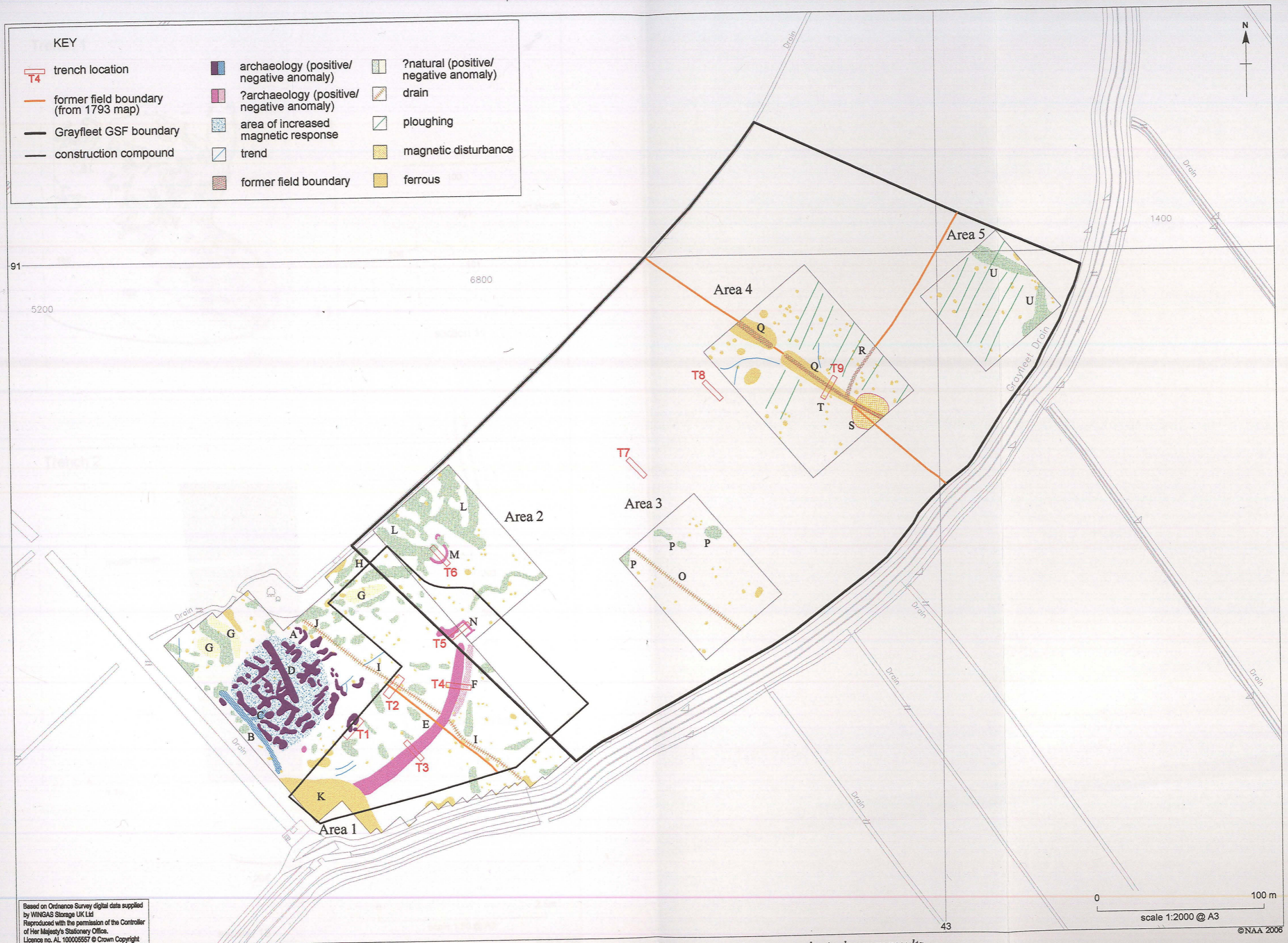
Figure 3 Grayfleet Gas Storage Facility: trial trench locations overlain on geophysical survey results
