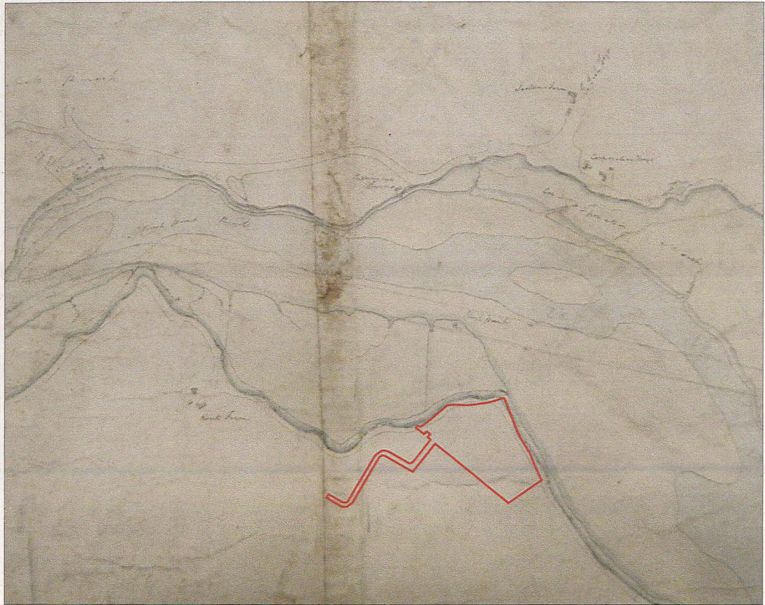
Figure 3: Map of Boston Haven dated 22nd April 1800 at approximately 1:10,000, with site outlined in red. Existing course of river depicted with proposed canalisation drawn in pencil
