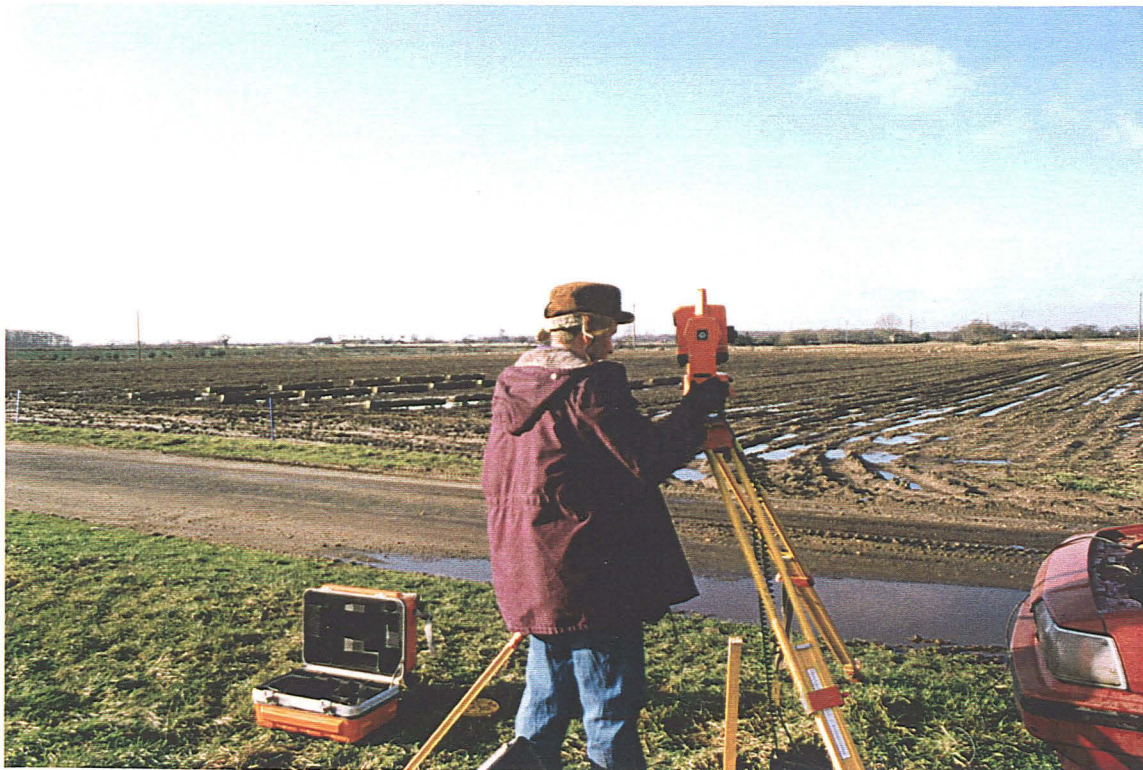
Pl. 4 Area 8 after walking. Looking SW from Area 2; setting up geodimeter in foreground.
