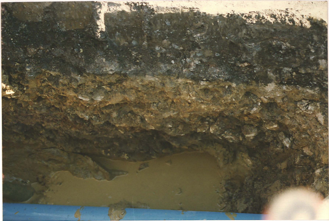
Pl. 19 Sequence of deposits at 22, showing a deposit of grey soil with peat 0.5m below the road surface. Beneath the peat was yellow and grey clay with sand.
