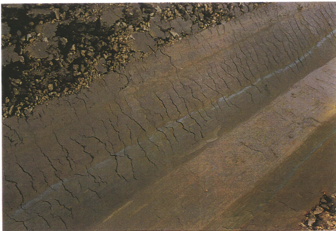
Pl. 3 Alluvium deposits visible in perimeter ditch.
