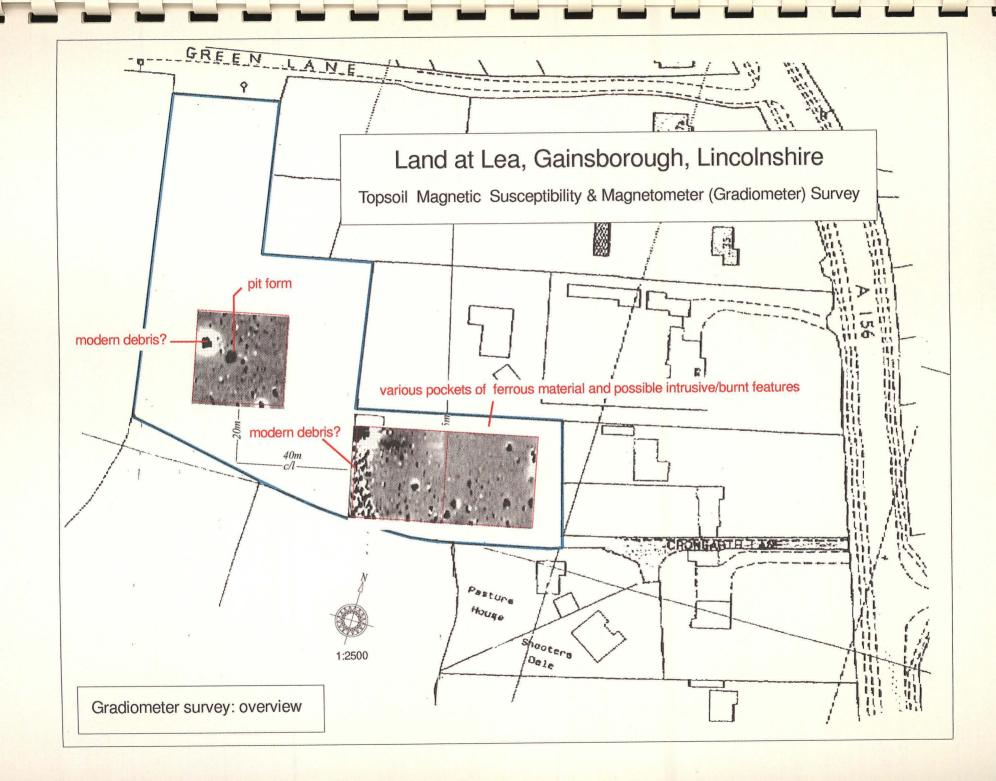
Topsoil Magnetic Susceptibility & Magnetometer (Gradiometer) Survey Gradiometer Stacked Trace plots
