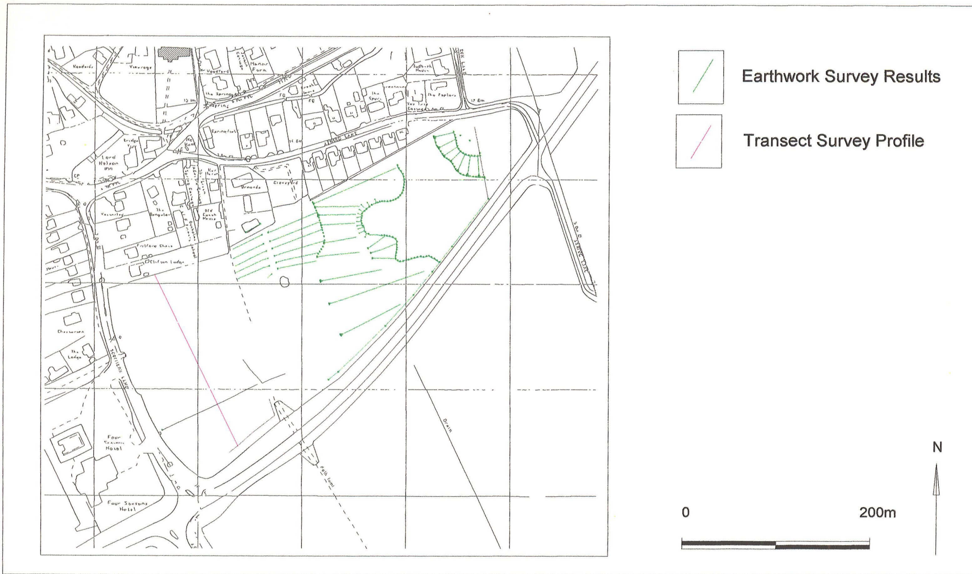
Figure 11 - Earthwork Survey Results
