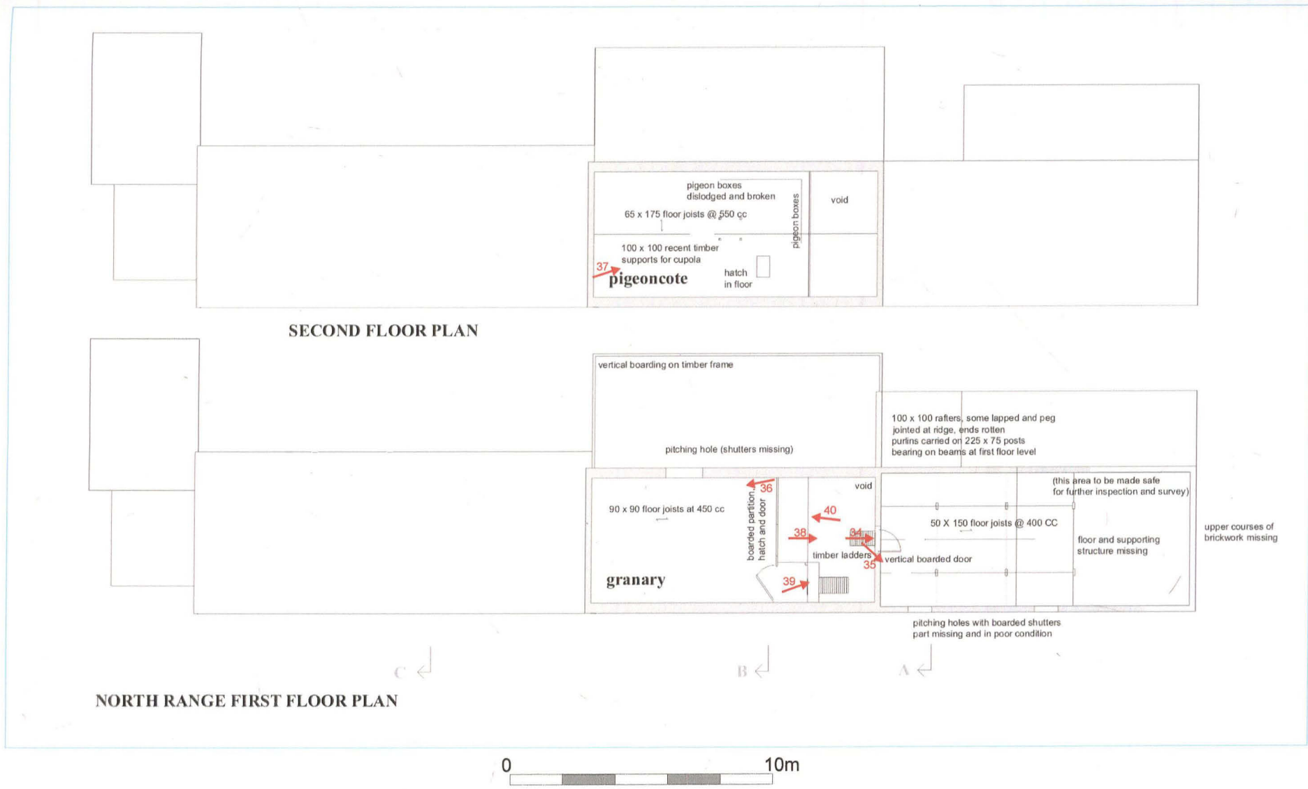
Figure 4: Plans of the first and second floors of the north range, as existing, with the plate number and position of photographs shown in red (listed in appendix 1) (scale 1:200).
