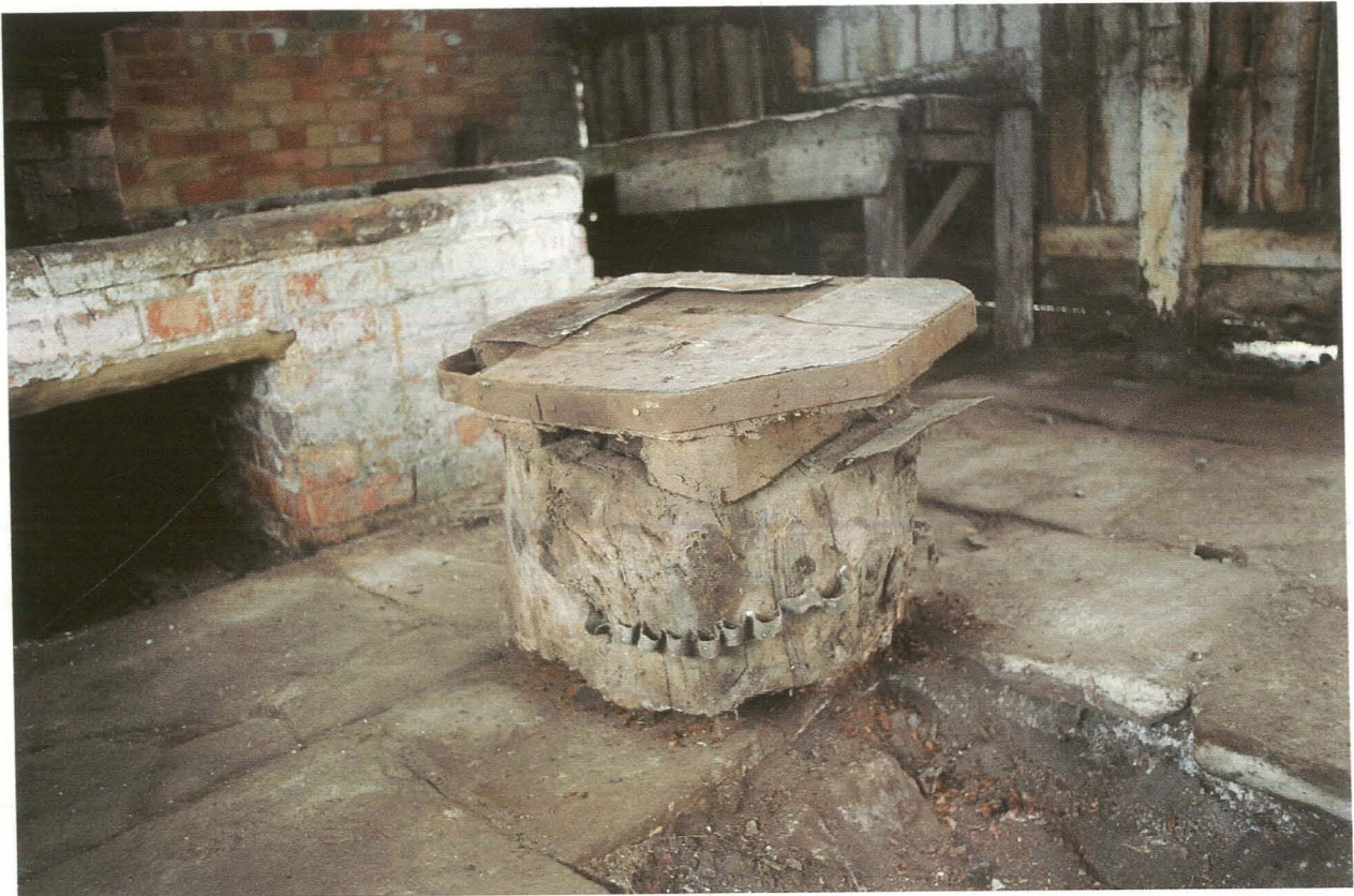
Pl. 17 Anvil base, next to original location marked by hole in ground . Note zinc metal strip nailed around the tree stump formed a crude tool holder.
