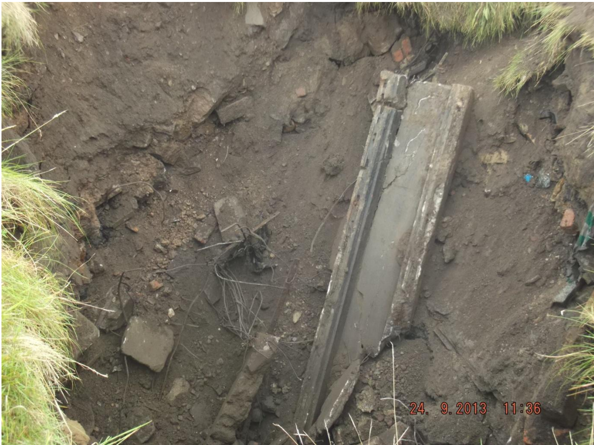
Illus 3 TP14 showing type of infill at south end of site
