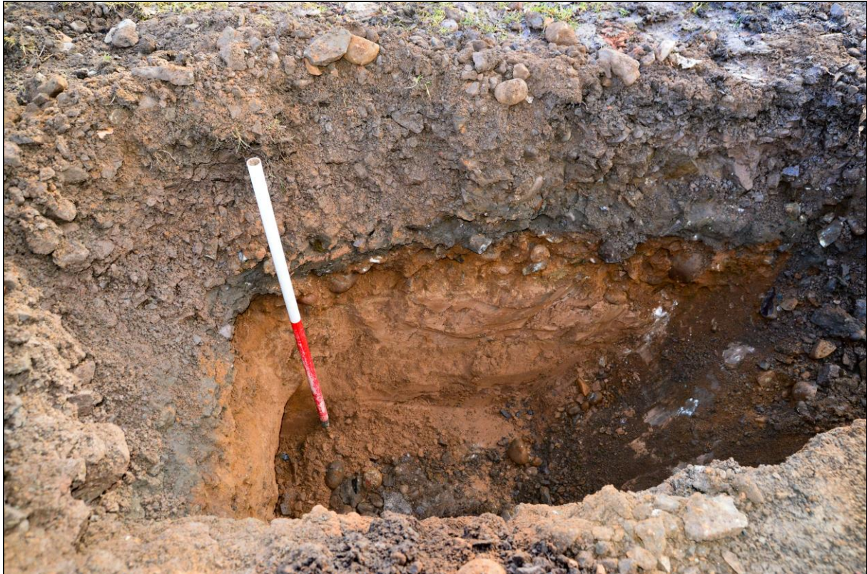
Illus 4: Stratigraphical profile of sump for Soakaway 4, indicating light brown silty overburden and deep underlying clean sandy deposit (orange/brown) separated by a dark, silty organic layer containing numerous small cobbles.
