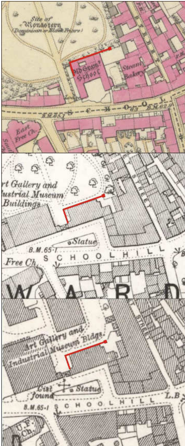
Illus 15 Ordnance survey maps with proposed substation base and cabling trench in red. (top) Aberdeen Sheet LXXV.11 (Old Machar) Publication date: 1869 (middle) Aberdeenshire 075.11 Publication date: 1902 (top) Aberdeenshire 075.11 (includes: Aberdeen) Publication date: 1926 (copyright National Library of Scotland).
