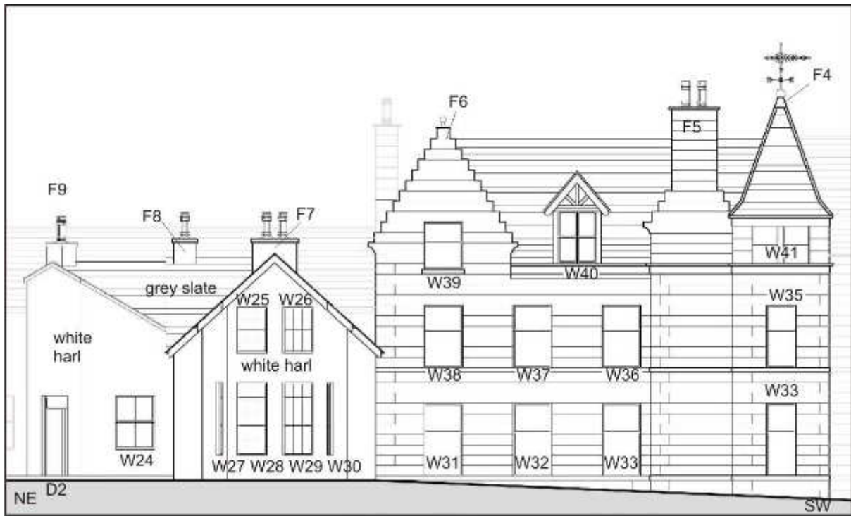
Illus 20 NW elevation annotated with feature numbers used in this survey (copyright Fitzgerald Associates)
