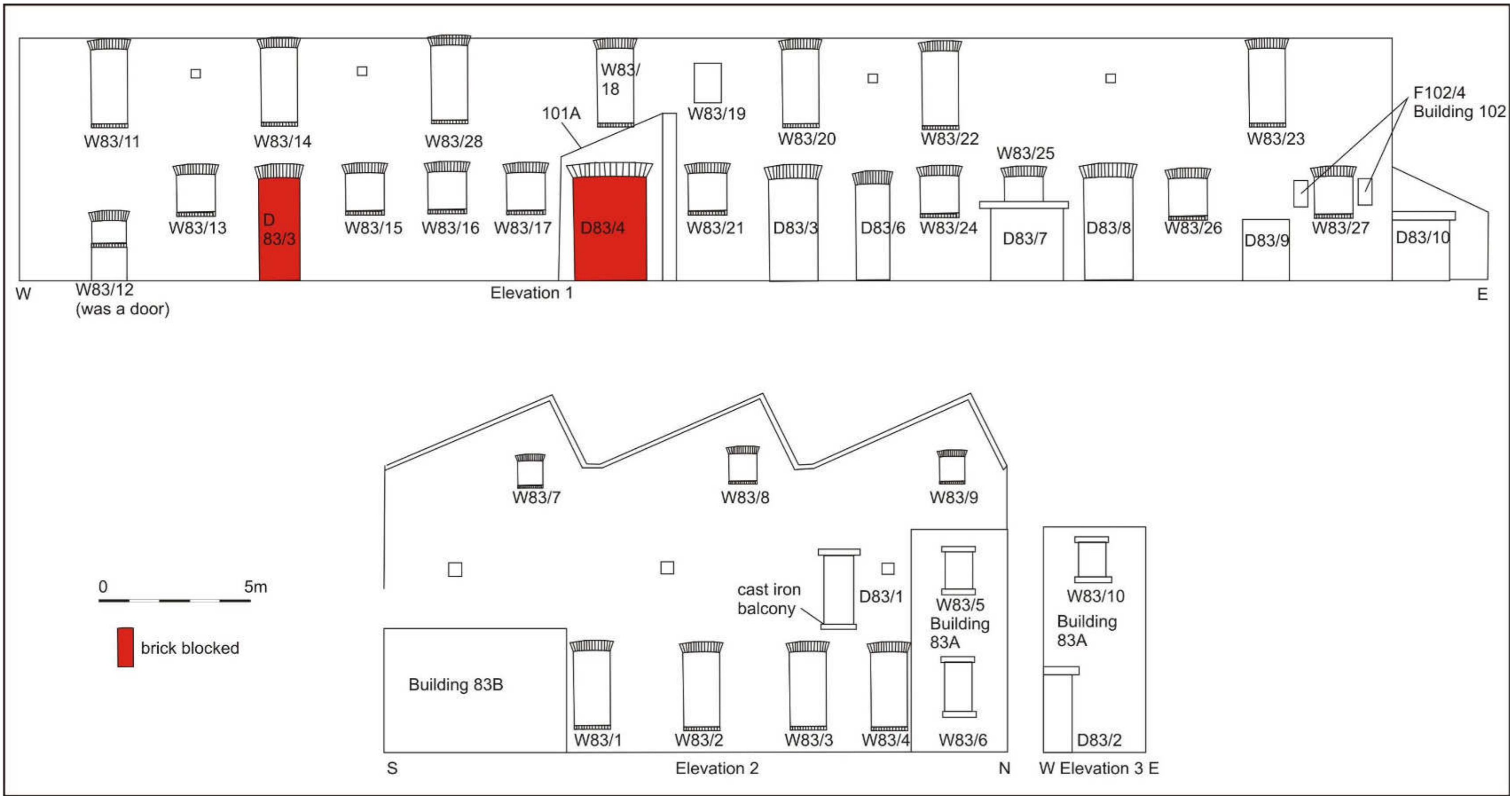
Building 83 S and E elevations annotated with feature numbers used in the survey
