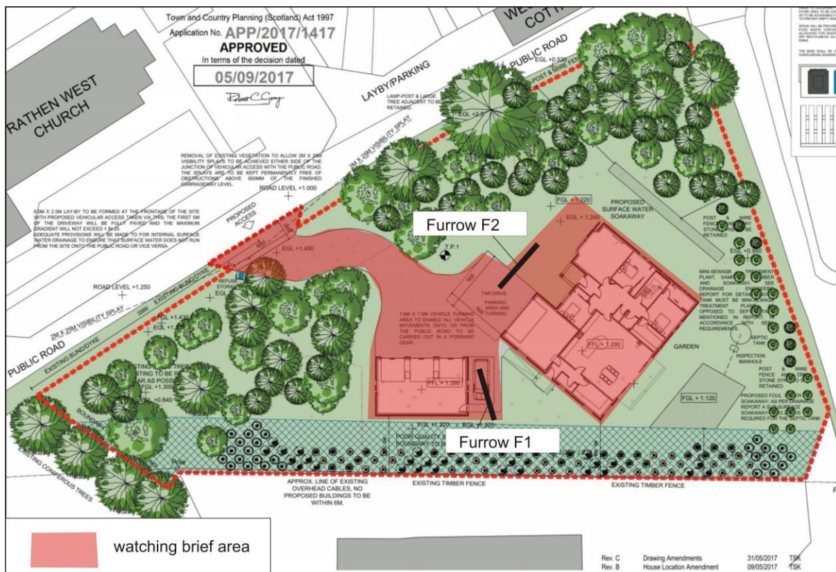
Illus 2 Site plan showing area of watching brief and furrows F1 and F2 (copyright Claymore Homes)
