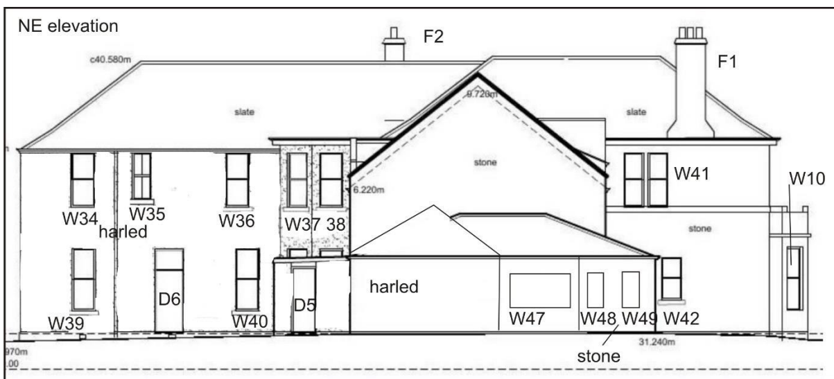
Illus 4 NE elevation with numbers used in this survey (copyright Fouin + Bell)
